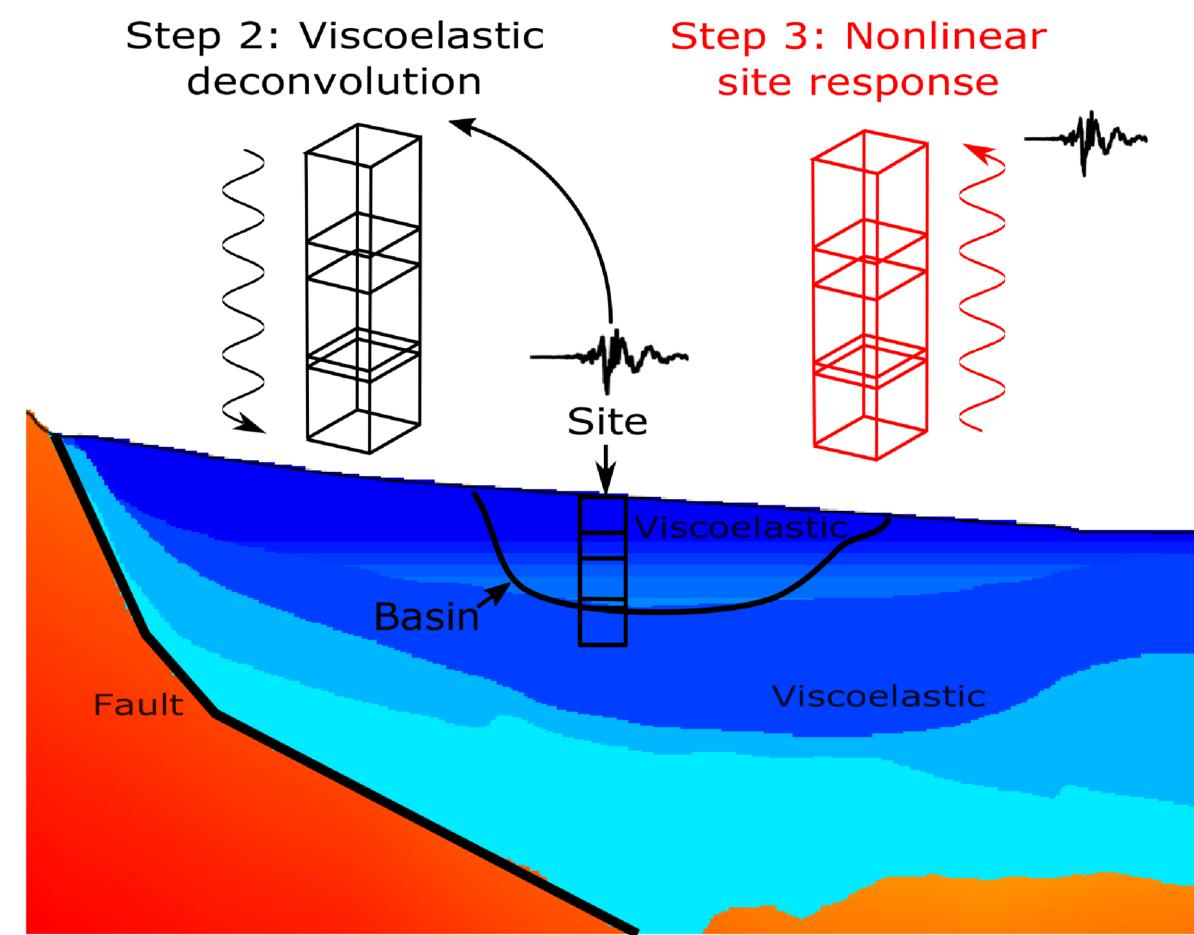
Step 1: 3D viscoelastic simulation
