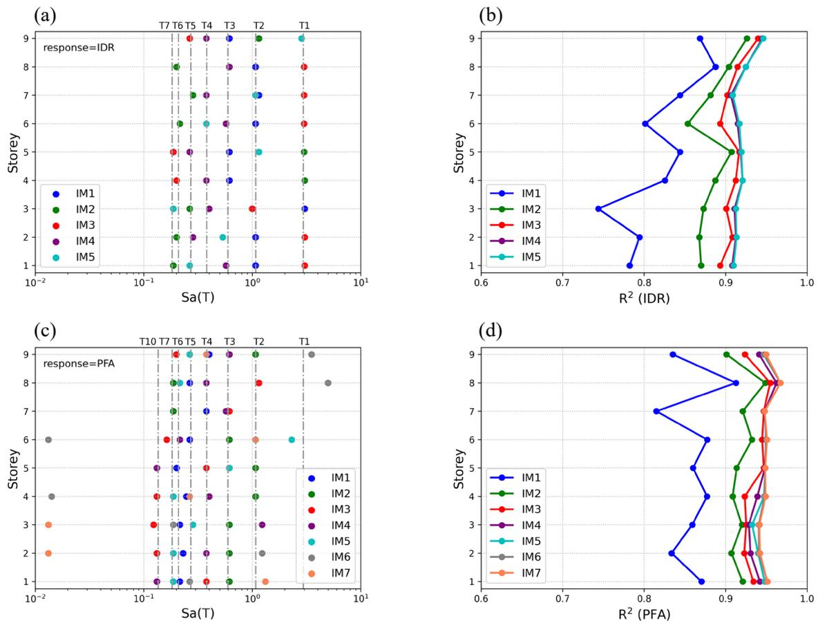
Figure 6: Variable selection and coefficient of determination ( $R^2$ ) for Building B a-b) IDR; c-d) PFA.
