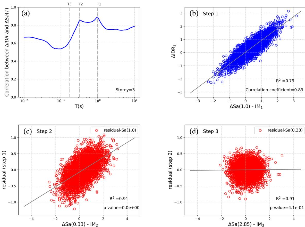
Figure 4: Variable selection procedure for IDR at Building A third storey a) correlation between  $\Delta IDR$  and  $\Delta Sa(T)$ ; b)  $\Delta IDR_3$  versus  $\Delta IM_1$ ; c-d) relation of residuals with the selected  $\Delta IM$  at steps 2 and 3.
