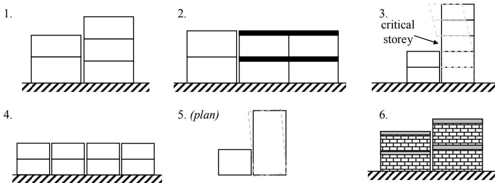
Figure 7.1 Critical pounding configurations
