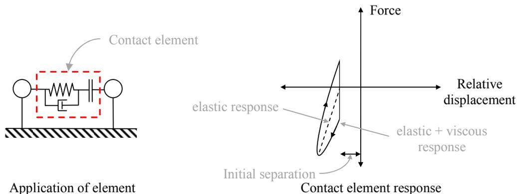
Figure 2.1 Linear contact element characteristics and application
