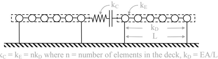
Figure 2.2 Optimum collision stiffness for multiple element object collisions
