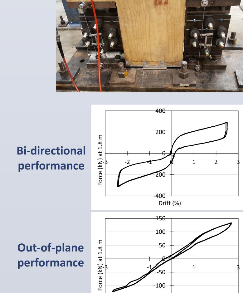
Figure 5. Bi-directional testing of the Nelson Column test
