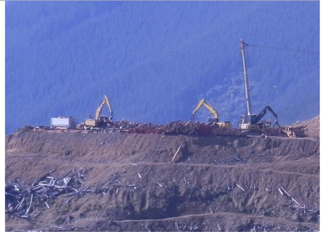
**Figure 9: Recovery during harvest (integrated biomass recovery): the hook-up bin is on the left, parked at the end of the truck lane and near the loader, so that the machine can easily intercept the offcuts disposed of during log fleeting.**
