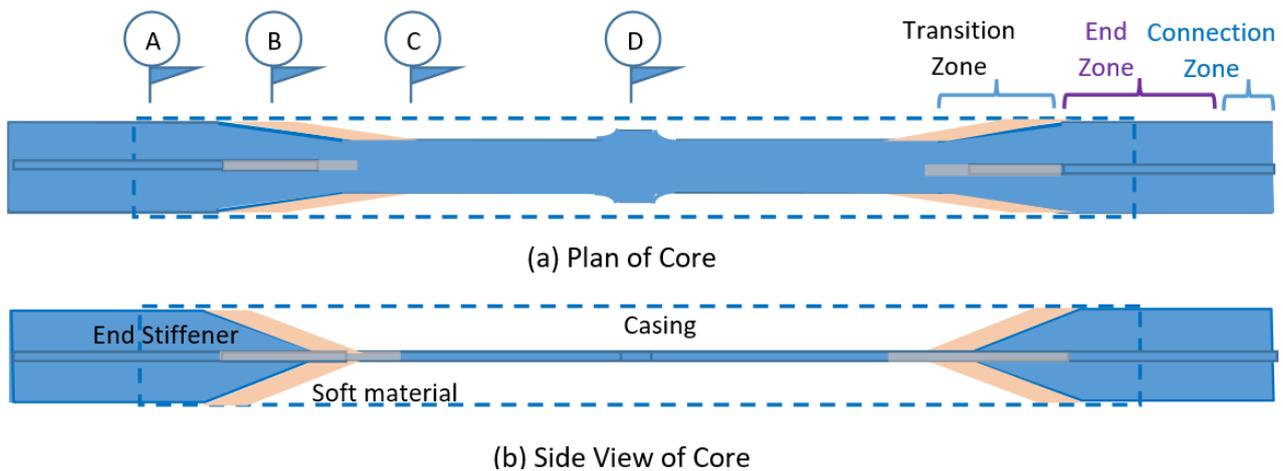
Figure 1. BRB Longitudinal View (Not to Scale)
