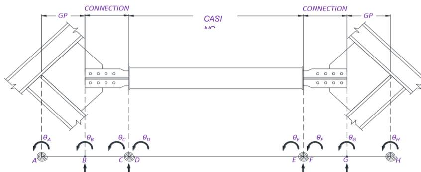
Figure 3. BRB System Sub-elements and Rotational DOFs (Westeneng, 2017)
