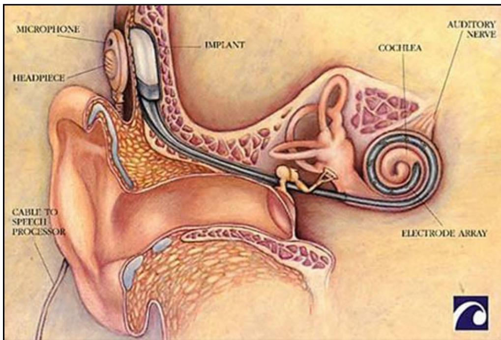
Figure 9: Diagram showing the insertion depth of a typical electrode array (1.5 turns) (Scottish Cochlear Implant Programme, 2008)
