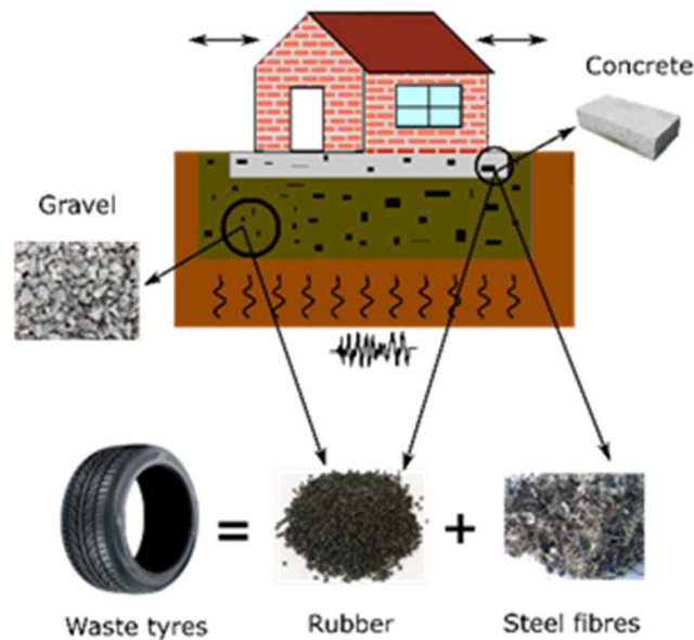
Figure 1. Eco-rubber seismic isolation foundation system.
