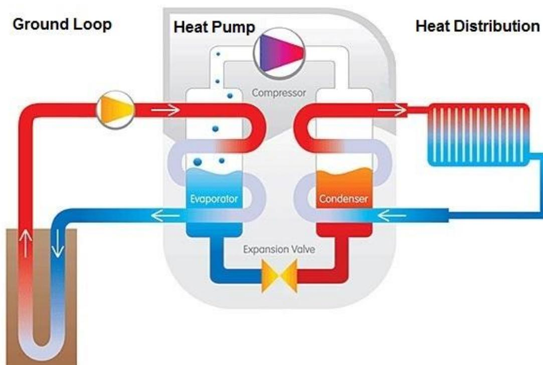
Figure 1: GSHP Schematic showing Ground Loop, Heat Pump, and Heat Distribution System. Image source: (5)
