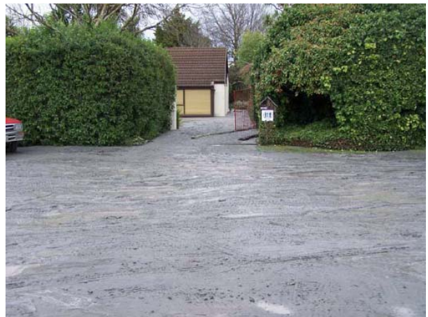
Figure 13. Manifestation of very severe liquefaction in residential area of North Kaiapoi; ~40 cm thick layer of silt-sand-water mixture covering a residential property affected by very severe liquefaction; the house suffered structural damage and large settlement
