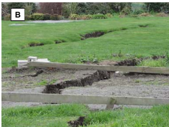
Figure 16. Large lateral spread cracks in farm land (positions A and B shown in Figure 15)
