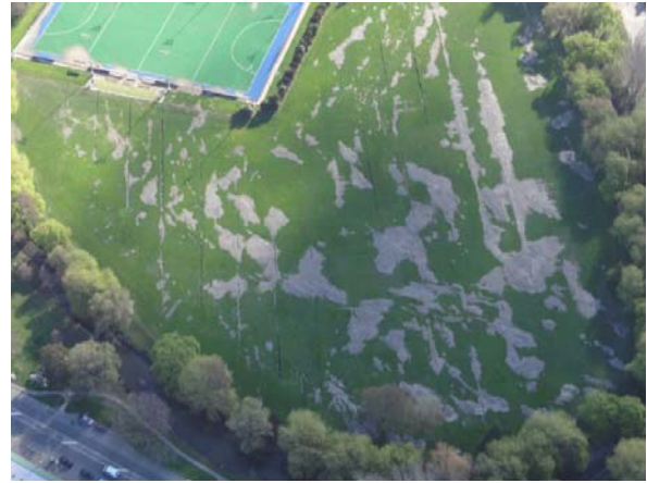
Figure 10. Evidence of extensive liquefaction (massive sand boils) in Porritt Park; using the vehicles (bottom of photo) or the hockey field (top of photo) for scale gives a good indication of the significant volume of sand ejecta
