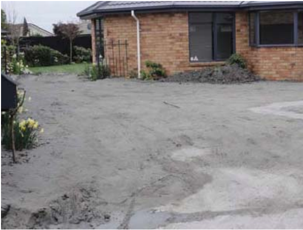
(a) Large volume of sand ejecta on residential land
