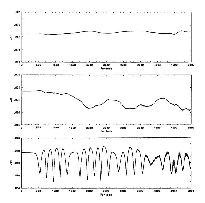
Figure 4. The time evolution of the resonant amplitudes  $a_{11}$ ,  $a_{42}$  and  $a_{93}$ , starting from the standing wave SAC with  $\epsilon=0.1$ .
