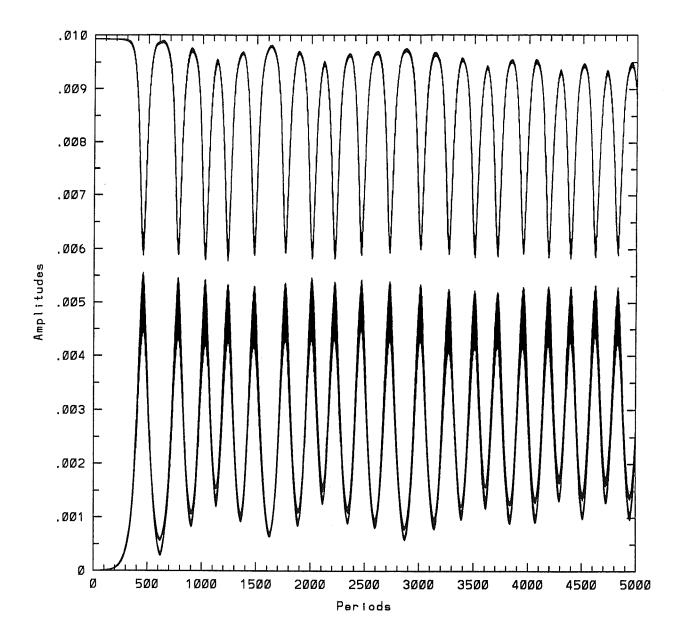
Figure 3. The time evolution of the resonant amplitude  $a_{93}$  at the top, then in order the two sideband amplitudes  $a_{83}$  and  $a_{10\,3}$  almost superposed, starting from the standing wave SNA with  $\epsilon=0.1$ .
