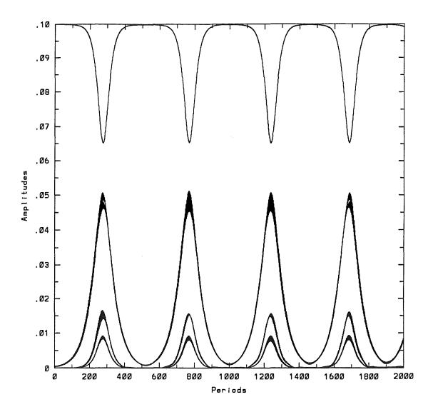
Figure 1. The sideband modulation of a set of 9 Stokes standing waves, where  $\epsilon=0.1$  for each. The cyclic recurrence in slow time results from the instability of the Stokes standing waves to a subharmonic disturbance. The fundamental amplitude  $a_{93}$  of each of the original standing waves is at the top, then in order the two sideband amplitudes  $a_{83}$  and  $a_{103}$  are almost superposed, followed in order by the sideband amplitudes  $a_{113}$  and  $a_{73}$ .
