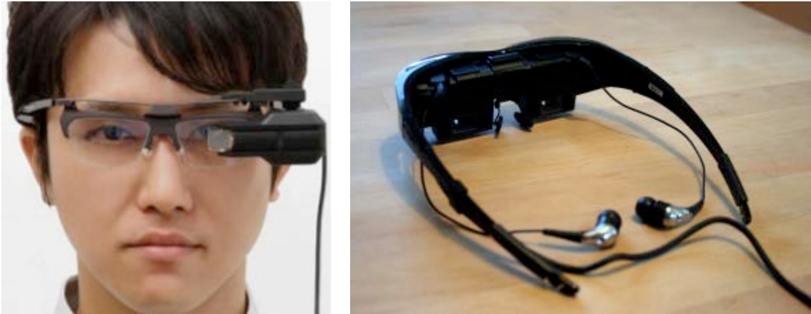
Figure 4.2: The Brother AirScouter and Vuzix HMD
