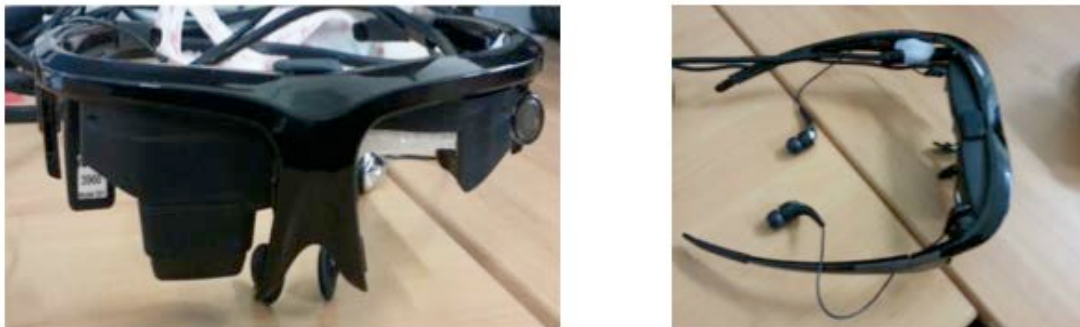
Figure 4.3: Modified Vuzix HMD
