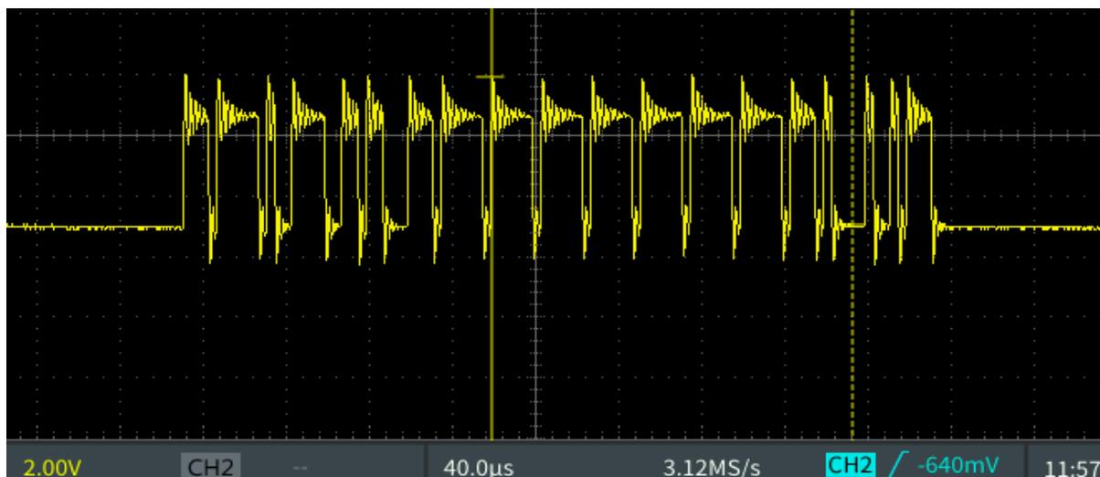
Figure 57 CAN High Signal.
