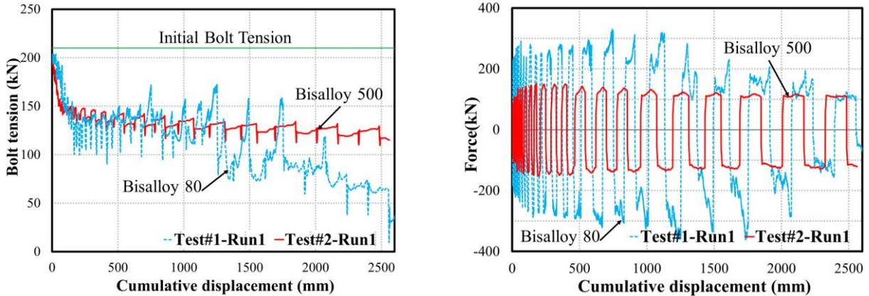
(a) The loss of bolt pretension force
