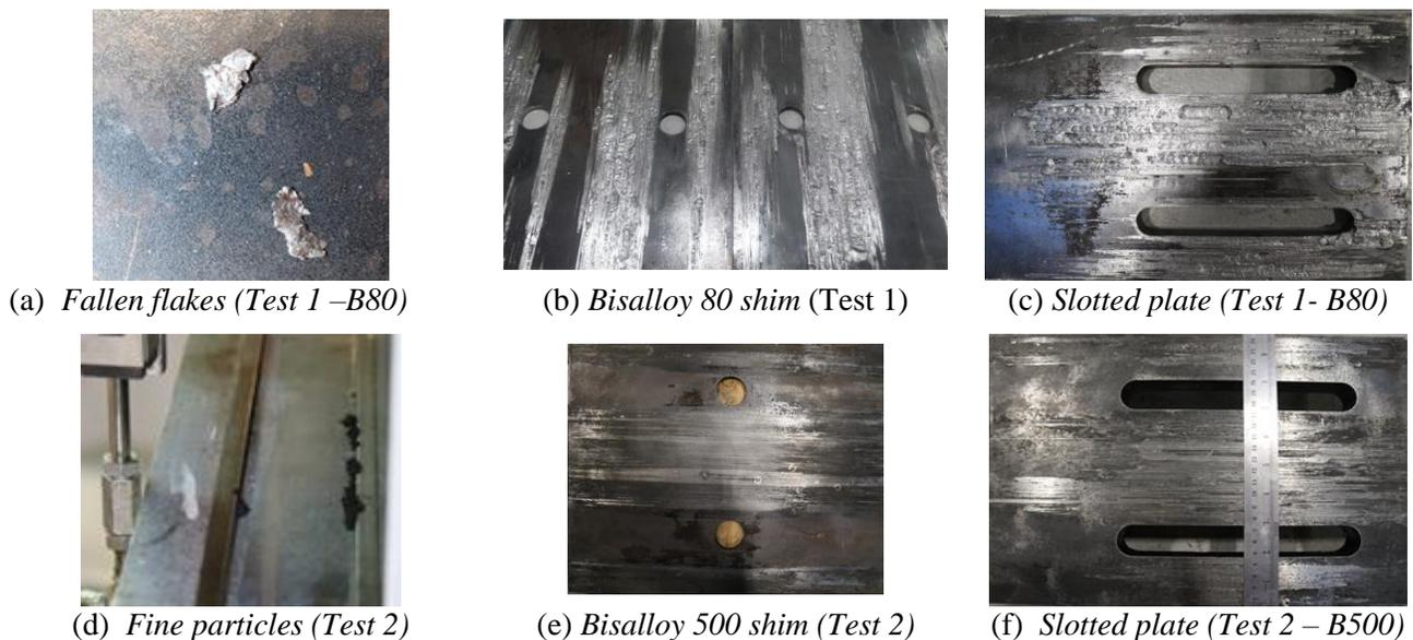
Figure 4. Tested plate surfaces and debris
