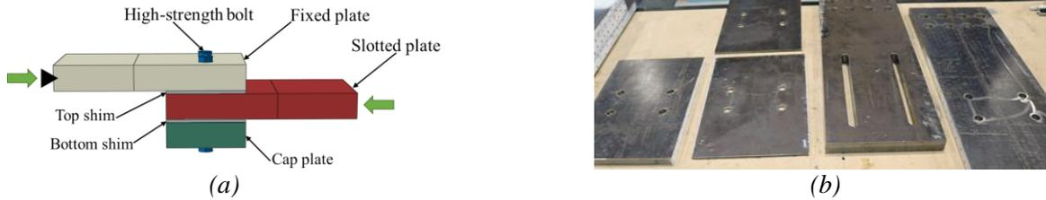
Figure 1. AFC. (a) assembled specimen (b) component; left to right: cap plate, shims, slotted and fixed plate
