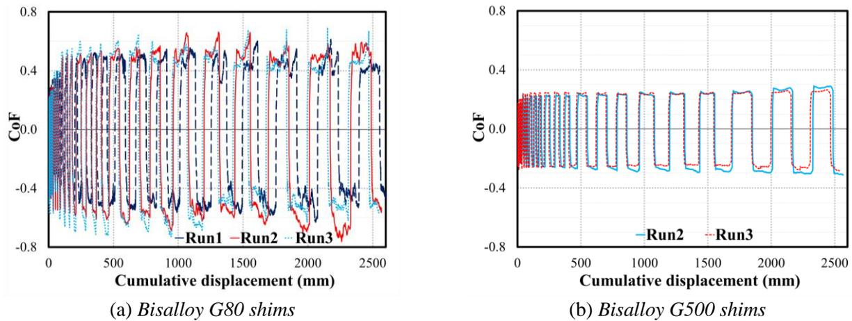
Figure 7. Friction coefficient AFC
