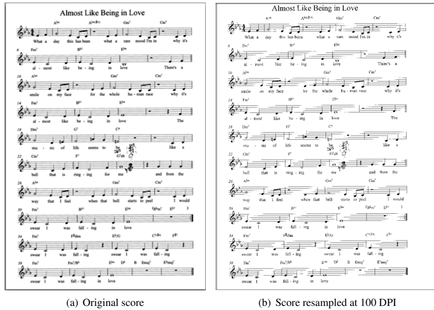
Figure 3.3: Low resampling resolution aliasing defect
