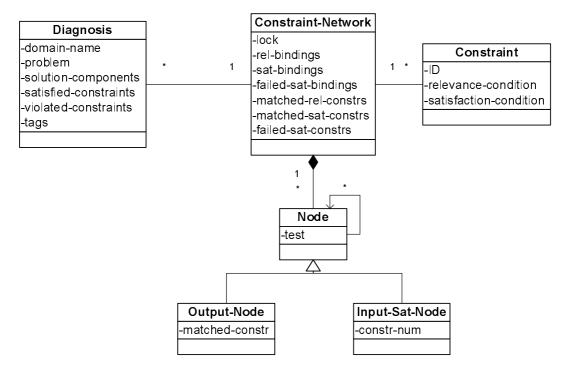
Figure 16. The class diagram for the Diagnostic Module
