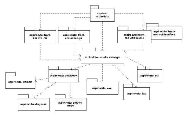
Figure 12. The package structure of ASPIRE-Tutor
