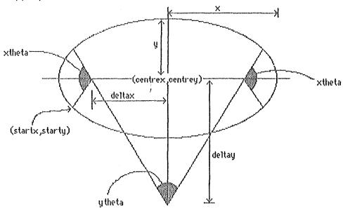
As can be seen, the starting point, the arc centres, radii, and degrees can all be calculated.
