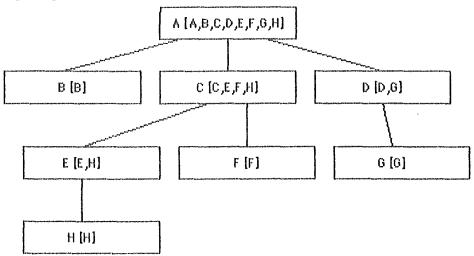
Each part of the object is labelled A, B, ..., H. The section labelled 'A' is the top of the object hierarchy. The labels within brackets at each level is a list of those sections which the "pointers to numbers" of that level can point to.
