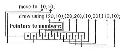
This idea could even be extended further whereby the object is represented as a string of graphic codes (terminal dependent) and the "pointers to numbers" point to the numbers to be transmitted within this string. This would mean that an object would only have to have its defining commands executed once, unlike the current animation where such must occur at each frame.
