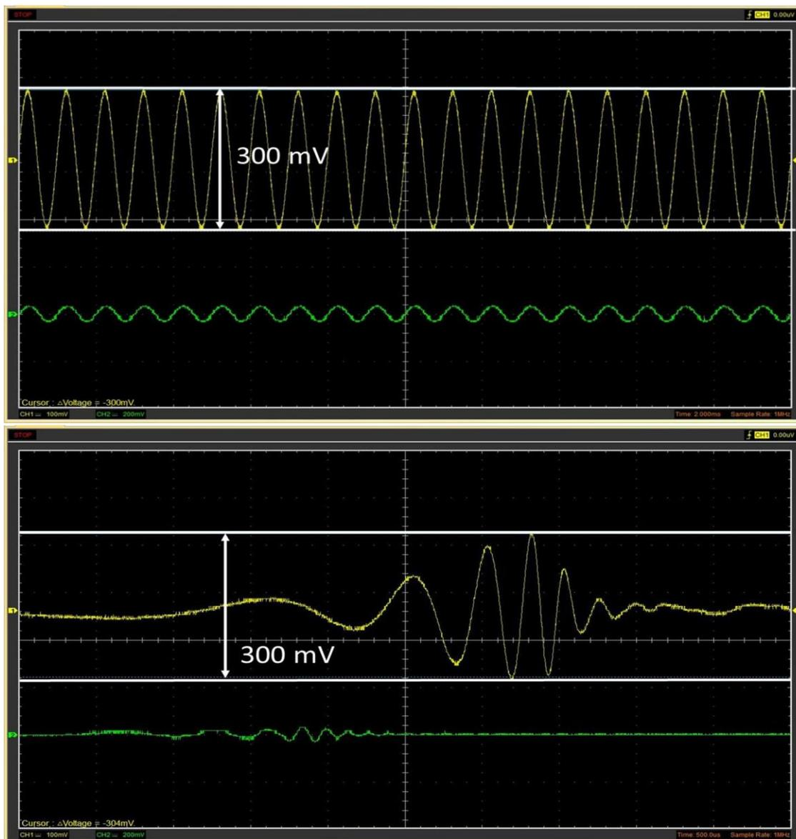
For a 90 dB SPL stimulus the reference tone attenuator value was set to 0.095 and the chirp attenuator value was set to 0.09. The reference and chirp input/output voltages are shown in Figure 15.
