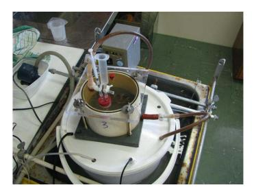
**Fig. 5.1** The system setup to measure the thermal tolerance range of fish acclimated to 8, 14 and 24°C.
