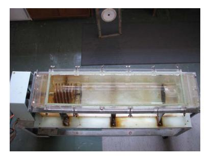
Fig. 4.1 Blazka-style swimming tunnel used for Ucrit experiments.
