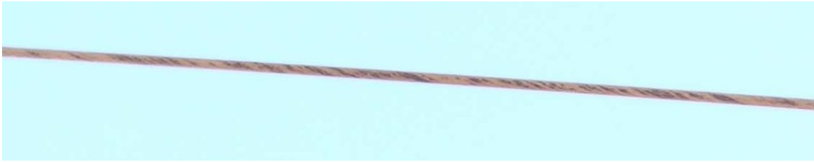
Figure 8 – Bungama transmission line conductor with a black substance apparently being emitted between strands.
