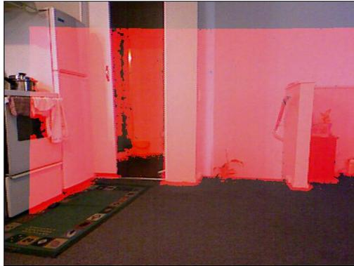
Figure 5.21: **Obstacle detection using Manduchi et al.'s algorithm.**
