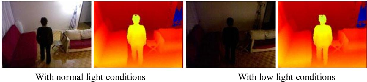
Figure 5.1: **Comparison of a video image with the corresponding depth map under different light conditions.** (Figure reproduced from [79]).
