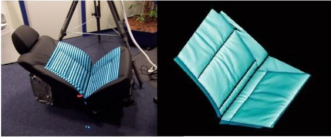
Figure 2.4: **3D survey of a car seat.** (Figure reproduced from [15]).
