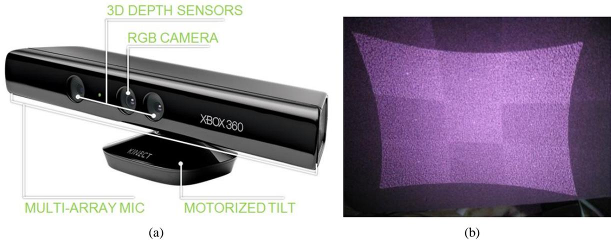
Figure 2.5: **Kinect sensor and its IR pattern.** (a) Kinect sensor. (b) Structured infrared pattern projected by Kinect depth sensors.
