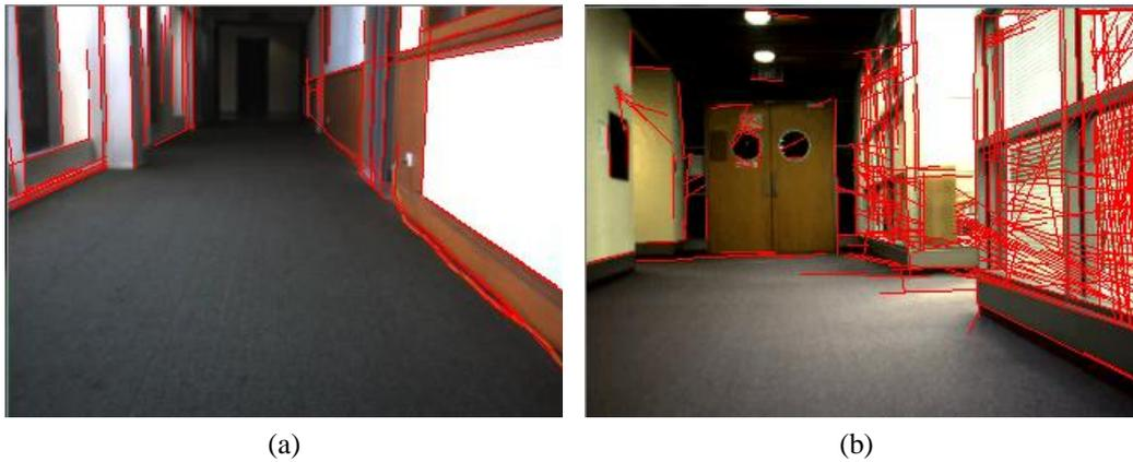
Figure 5.13: **Result of the Canny edge detector and the Hough Transform.**
