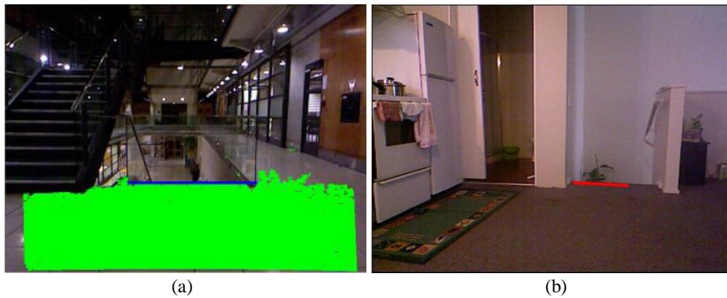
Figure 5.27: **Drop-off detection.** (a) a drop-off line is detected shown in blue colour. (b) only part of the drop-off is detected.
