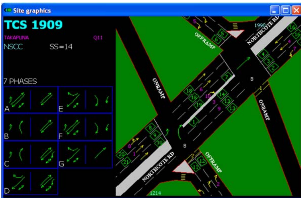
Figure 10: Northcote Interchange and SCATS® Detector Layout
