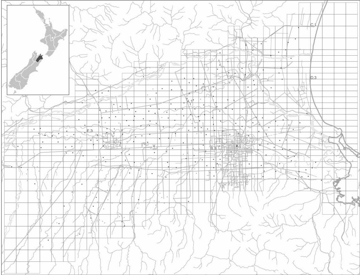
Figure 1. Map of Marlborough, showing wells, the MODFLOW grid, rivers, and roads. The coast is at the right side. The city of Blenheim is a bit right of middle. The labels A1, B3, C1, D3, and E3 are environmental control points, with their MODFLOW layer. The small gray dots correspond to the lowest volume wells, which were fixed in the simulation and optimization. The larger black dots are wells that trade. The inset shows Marlborough highlighted within New Zealand.
