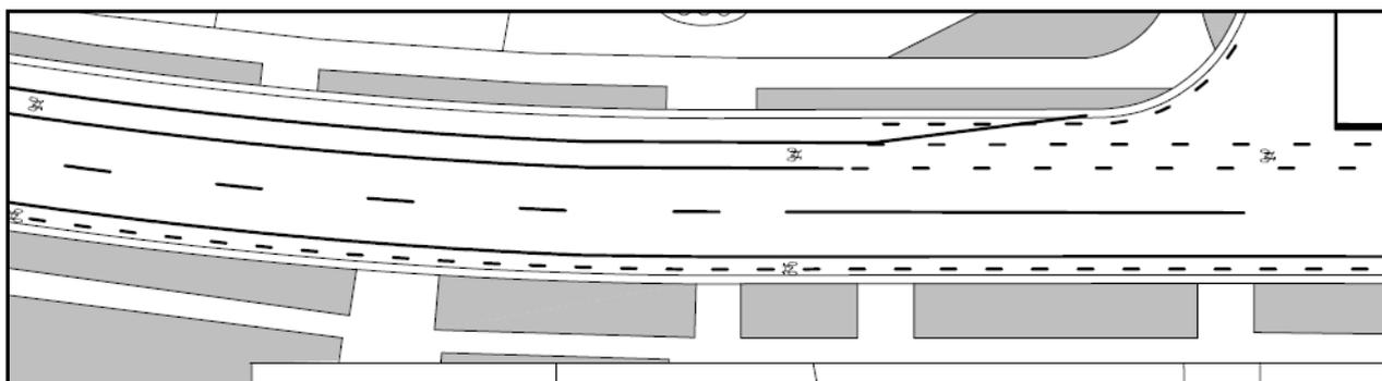
Figure 1: New Brighton Road -Typical Mid-Block Cycle Lane layout investigated
