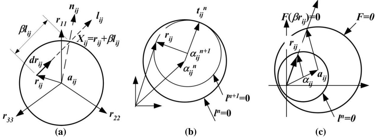
Figure 1 Geometrical interpretation of the model; (a) location of the conjugate point,  $X_{ij}$ , plastic shear strain increment direction,  $n_{ij}$  and stress increment direction,  $l_{ij}$ ; (b) hardening rule with respect to general loading surfaces; (c) hardening rule of the virgin or the first loading surface,  $n=1$ .
