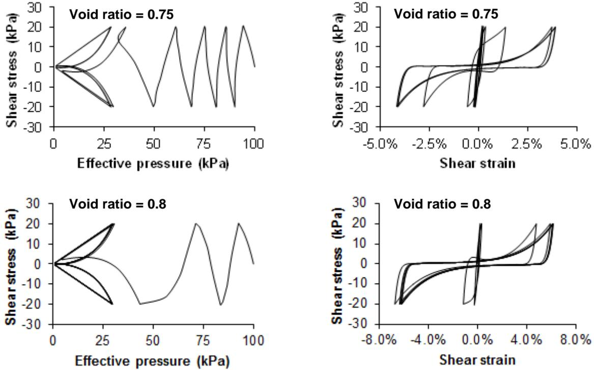
**Figure 2** Strain controlled simulation of Toyoura sand for void ratios of 0.75 and 0.8 under identical bi-directional shear strain cycles of  $\epsilon_{zx}$  and  $\epsilon_{yz}$  conforming to the torsional stress path ( $b=0.5$ ) with  $\eta=0.2$  and  $p=100\text{kPa}$  using the model parameters available in [1]; the shear strain is defined the same way as the generalized plastic shear strain, but with the total strain tensor
