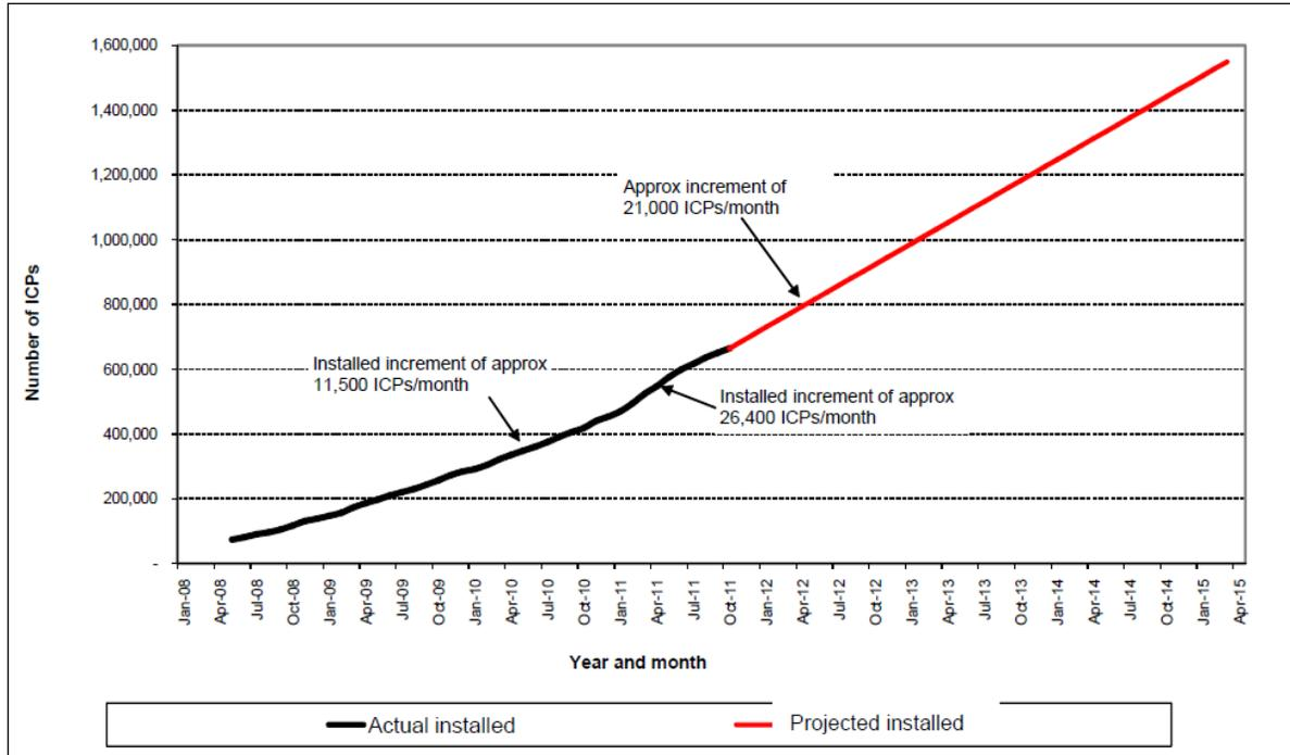
FIGURE 1: ESTIMATE OF ACTUAL AND PROJECTED AMI METER INSTALLATIONS
