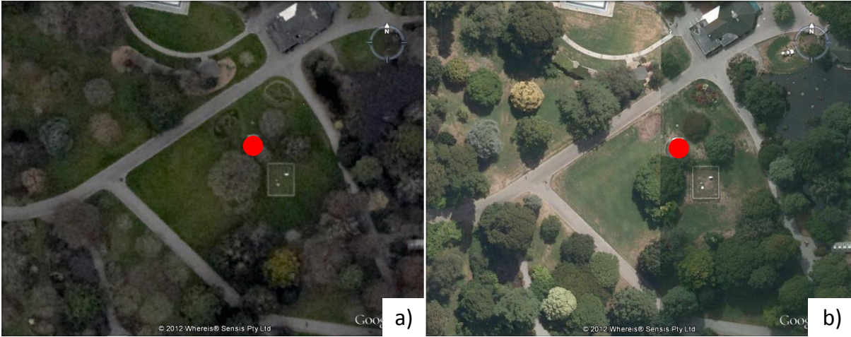
Figure 2. CBGS liquefaction surface manifestation a) Darfield earthquake; b) Christchurch earthquake
