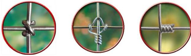
**Fig. (2).** Selection of knots used in the fabrication of rectangular netted wire fencing. From left: stiff-stay, fixed, and hinge-joint knot. Each knot has its own unique characteristics which see them used for different applications. These knots require dedicated tooling and hence consideration at the early stages of the design of the machine. (Image courtesy South Fence Machinery (New Zealand))
