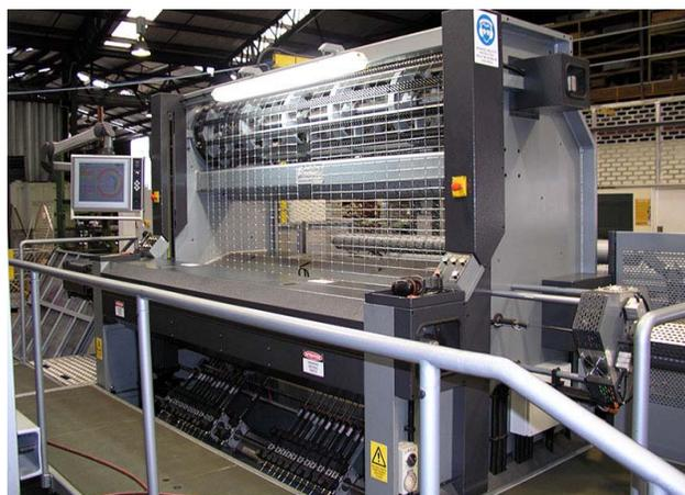
**Fig. (1).** Example of a specialised machine for knitting wire fences. Various knot types are available: this particular machine produces a fence with a 'stiff-stay' knot. The image hardly does justice to the size, complexity, and engineering precision of these specialised machines. This particular machine is designed and manufactured by South Fence Machinery (New Zealand). (Image used by permission of that firm).
