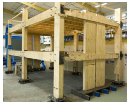
Figure 1: 2/3 rd scale post-tensioned structure for seismic testing research at the University of Canterbury
