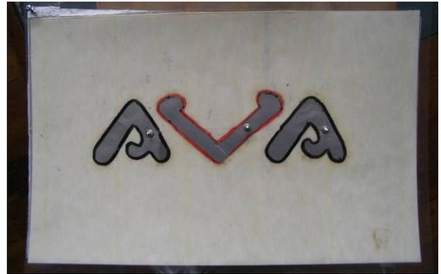
Fig. 6: LAD designed to discharge within lamination.
