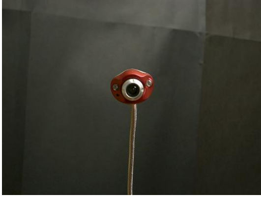
Figure 2: The webcam with infrared backlight used in this project.
