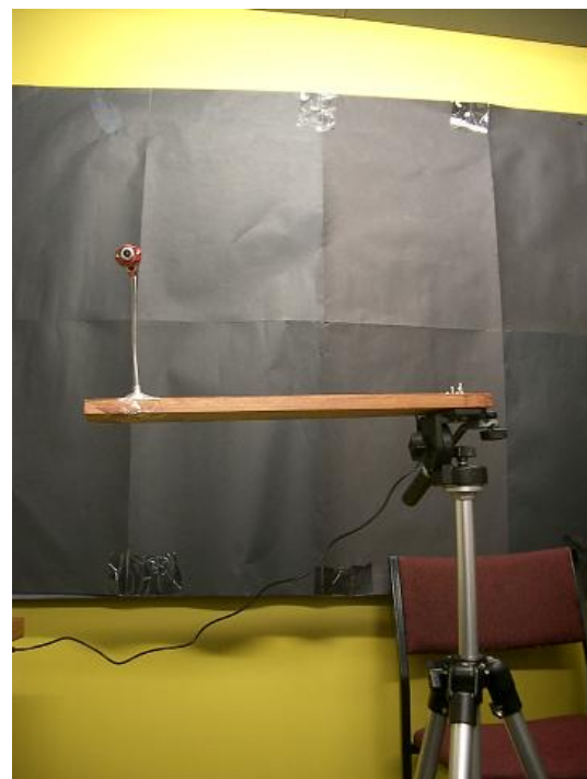
Figure 1: Physical setup of the marker based facial tracking system.
