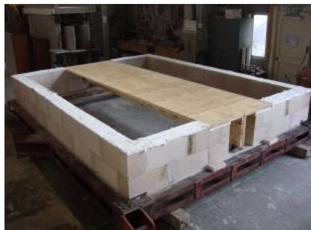
Figure 3: Beam type floor on the loading frame
