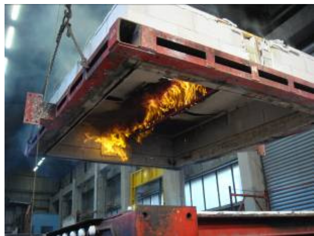
Figure 5: The underside of the beam floor directly after furnace testing
