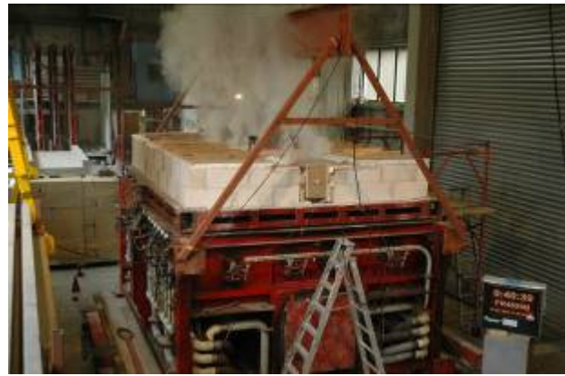
Figure 2: Furnace test of a timber composite floor at the BRANZ facilities
