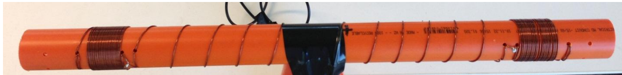
Figure 46: The Helical 27MHz antenna chosen for prototype construction.
