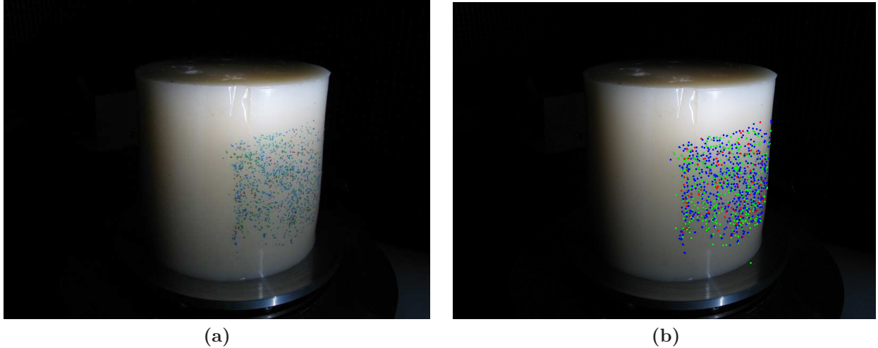
Figure 3. (a)Silicone gel phantom with coloured speckles. (b) detected red, green, and blue points.
