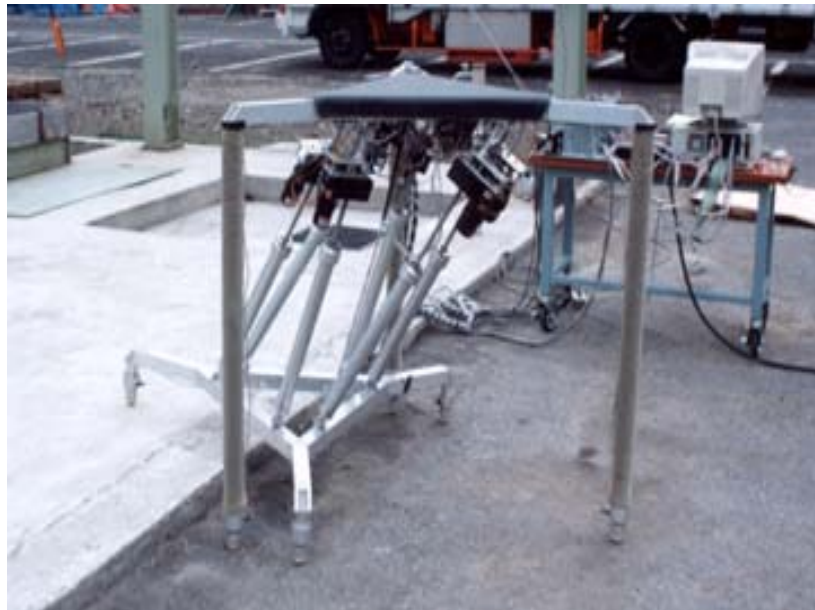
Figure 3.1. A walking machine with Stewart Platform
