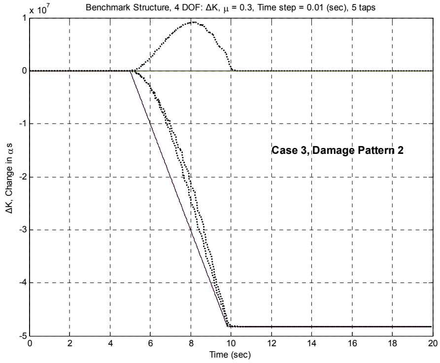
Figure 63 Case 3 and damage pattern 2 using the Two Step Method due to gradual failure
