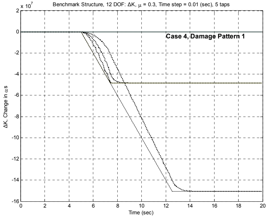
Figure 69 Case 4 and damage pattern 1 using the Two Step Method due to gradual failure
