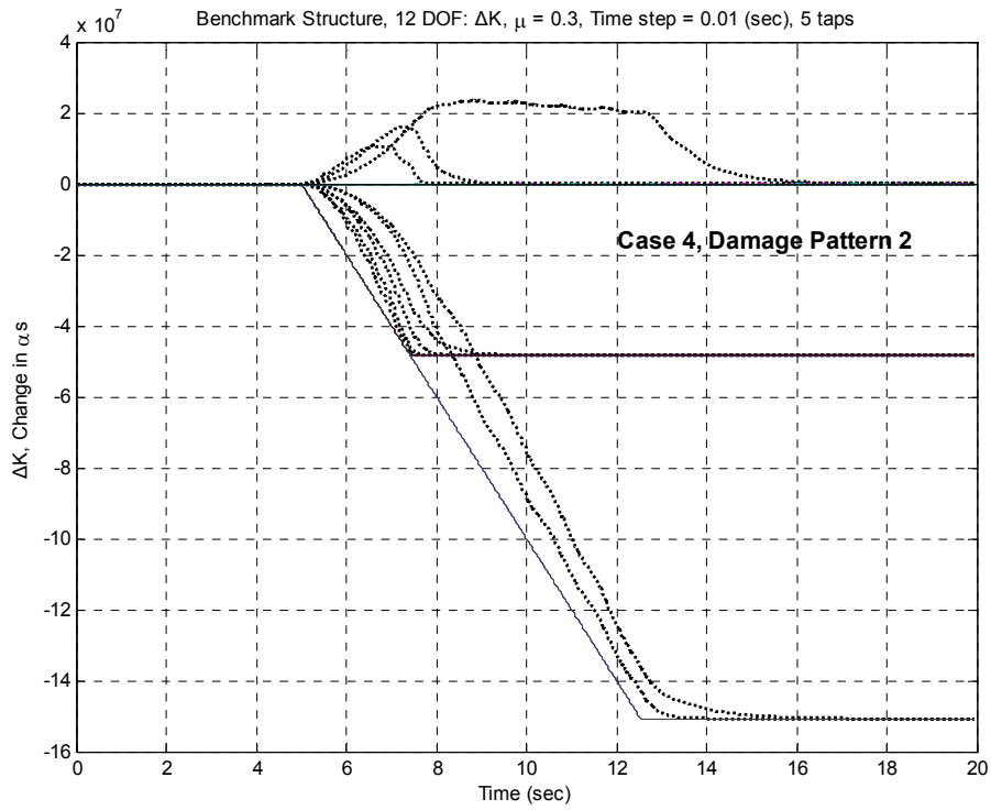
Figure 71 Case 4 and damage pattern 2 using the Two Step Method due to gradual failure
