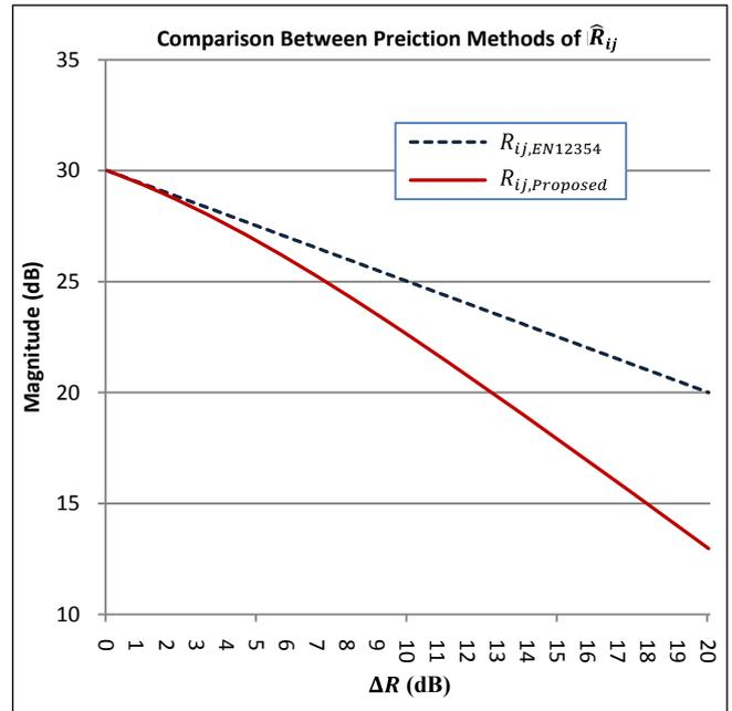
Fig.1 Comparison between  $R_{ij,Proposed}$  and  $R_{ij,EN12354}$  where  $R_{ij} = -10 \log \tau_{ij}$  and  $\Delta R = 10 \log \left( \frac{\tau_{ji}}{\tau_{ij}} \right)$ . The initial value of the calculations was set to  $R_{ij} = R_{ji} = 30$ dB.
