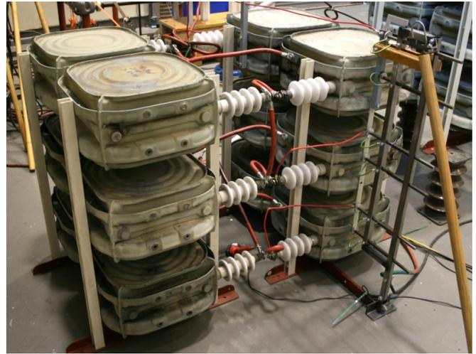
Fig. 3: One capacitor stage (with earthing lever applied).
