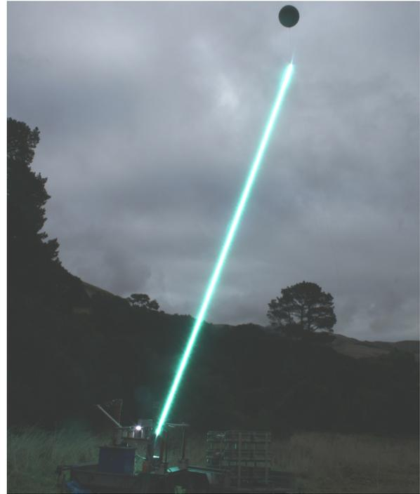
Fig. 1: A 10 m plasma path, created vertically to a weather balloon, used for outdoor atmospheric studies.
