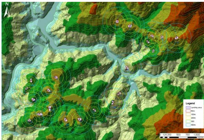
Figure 5: GIS map showing landing locations. The circles shown around the landings were used to determine average surrounding slope at different radii. Note that landings on top of the hills are generally larger than those mid-slopes (Figure prepared by Hamish Berkett).
