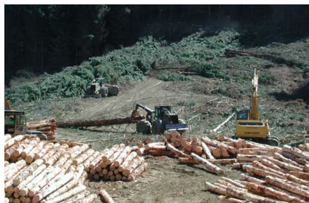
Figure 4: Mechanised processor located more centrally on the landing to minimise fleeting distance.
