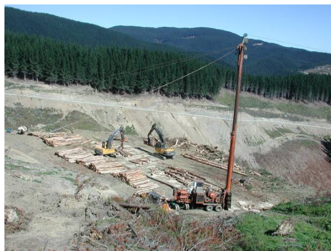
Figure 1: A typical (cable yarder) skid that incorporates the extraction, processing and loading phases of the operation.
