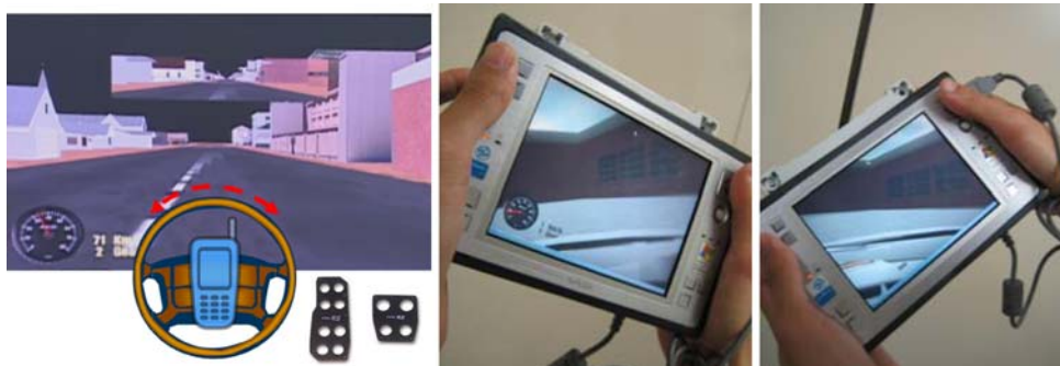
Fig. 9 Motion gesture recognition for the car driving metaphor. Roll rotation for direction handling and forward/backward movement for accelerator pedal control. An implementation is done using an UMPC (for simple gestures, a mobile phone implementation is possible, too)
