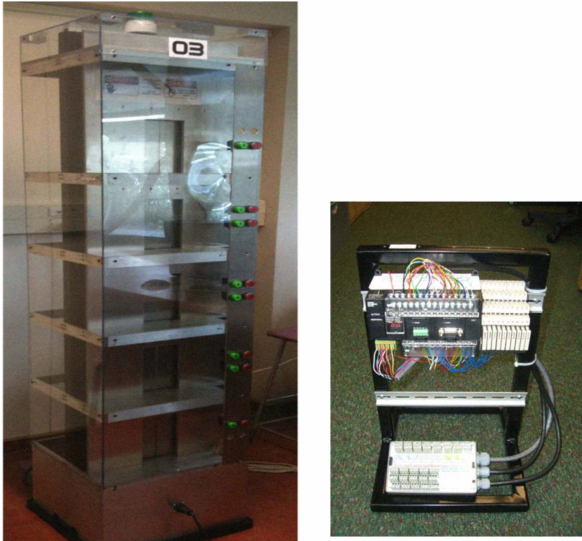
Figure 2. Elevator control project: the five-storey model elevator (left); and PLC as a control platform (right).
