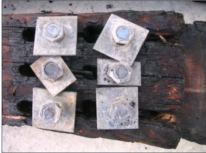
*Figure 8 Condition of W-W-W bolted connection after fire tests*
