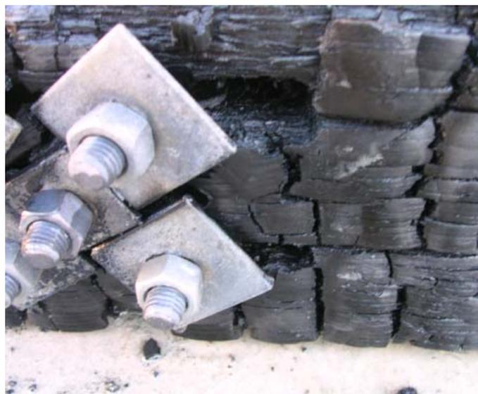
*Figure 10 Failure mode of W-S-W bolted connection after fire tests*
