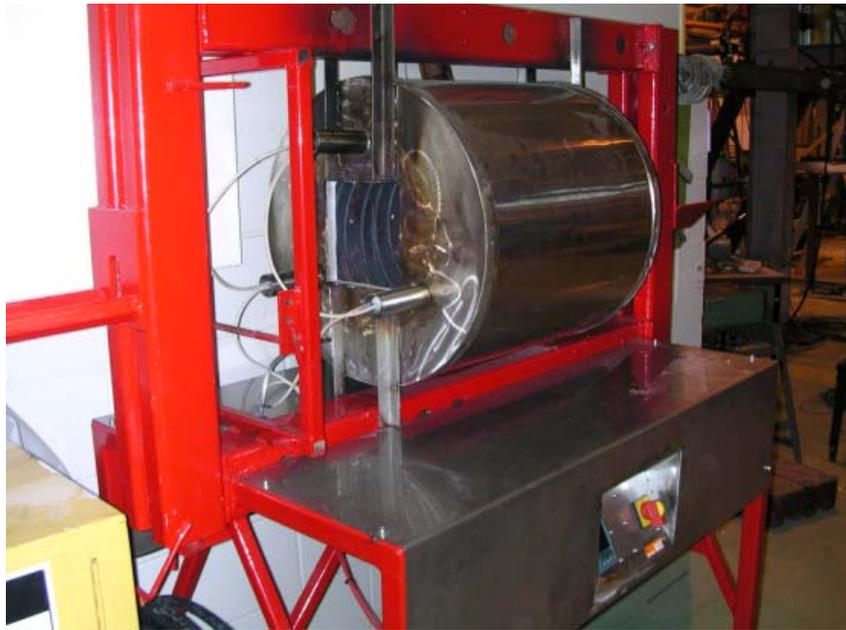
Figure 6 The test frame and furnace used for fire testing
