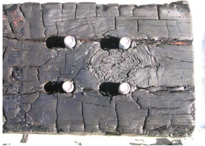
*Figure 9 Failure mode of S-W-S bolted connection after fire tests*
