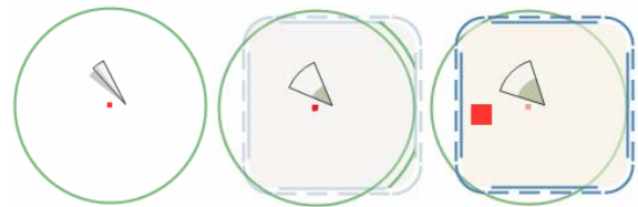
Figure 5: Pressure-Activated Lens. (left to right) As the pressure applied through the stylus increases, the lens gradually appears. After a threshold is reached, the lens becomes active.
