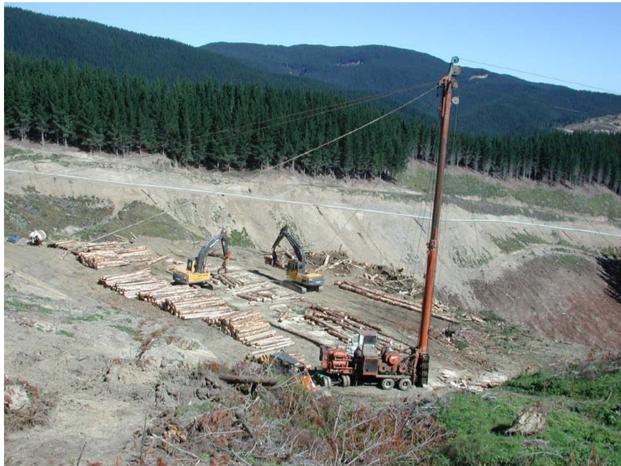
Figure 1: a typical NZ yarder landing – this one is 2950m 2 in size.
