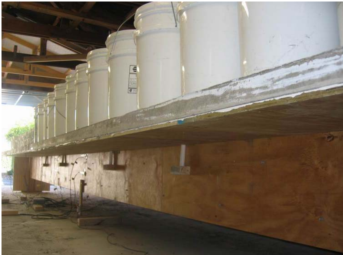
Fig. 6-6. Floor beam specimens loaded with buckets of water in the garage
