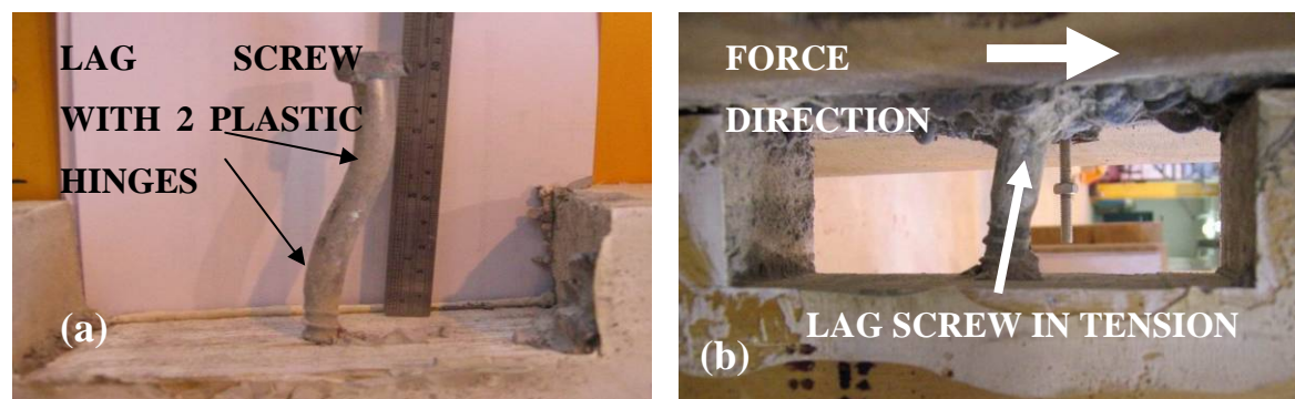
Fig. 4-5. (a) Formation of flexural plastic hinges in lag screw; and (b) Lag screw under tension in the direction of force
