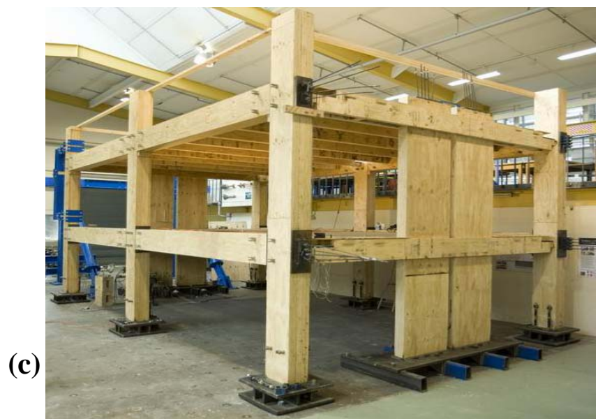
Fig. 2-16. Semi-prefabricated TCC floor system in New Zealand (a) Schematic diagram; (b) Erection of floor units; (c) Floor units in building frame (Yeoh et al, 2009a; Chapter 7)
