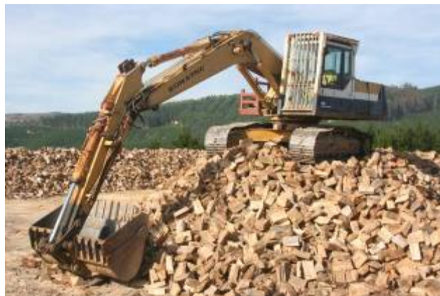
Figure 6: Excavator with a tined bucket, used to both pile for drying, as well as load out firewood.
