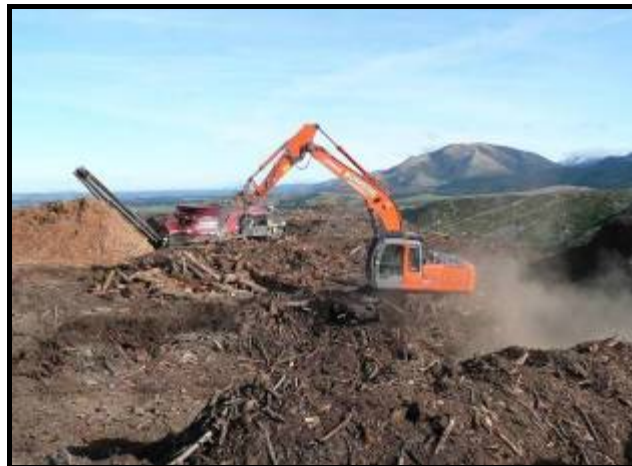
Figure 2: The excavator retrieving and piling the larger residue. The pile would then be hogged through the tub grinder.
