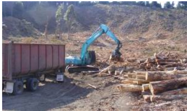
Figure 3: Recovering biomass from the landing and cutover and loading it into a bin truck.
