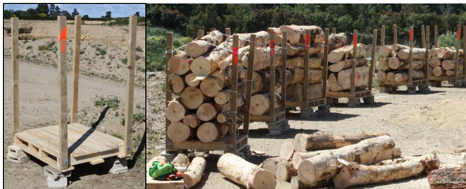
Figure 8: One of the 12 pallets with fitted uprights situated on cinder blocks; and pallets being loaded with logs prior to covering.
