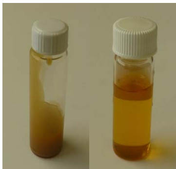
Figure 5-6 Oil product from low (left) and high (right) reflux processes.
