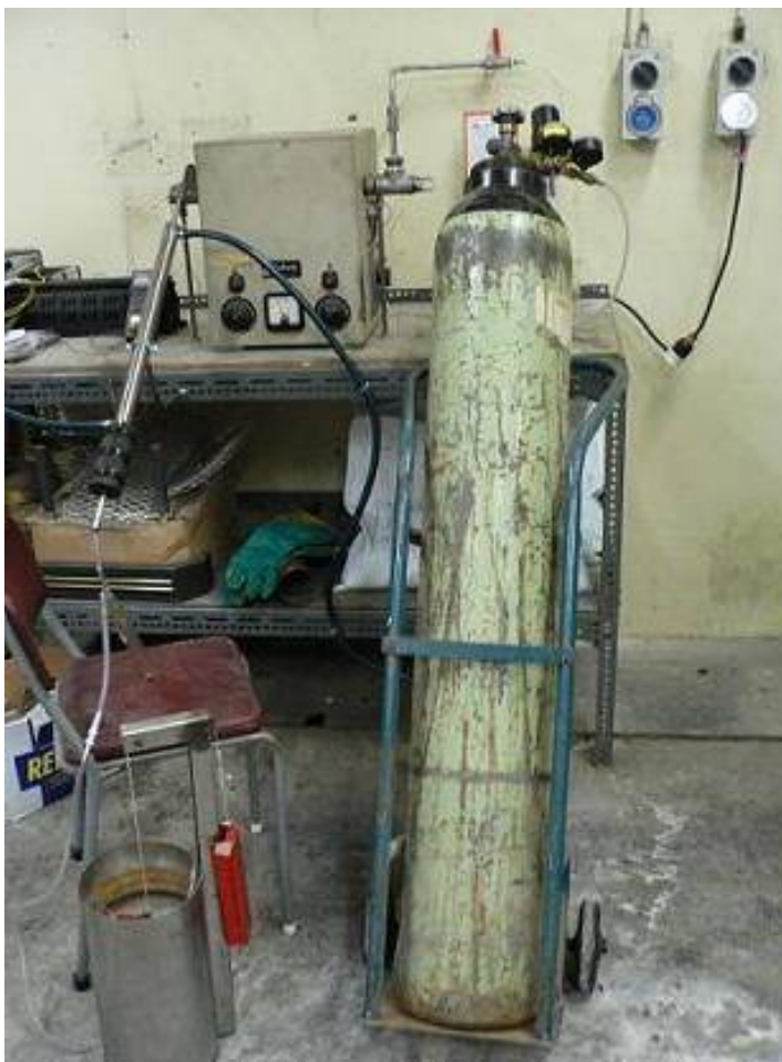
Figure 4-1 Scheme and picture of horizontal pyrolysis apparatus
