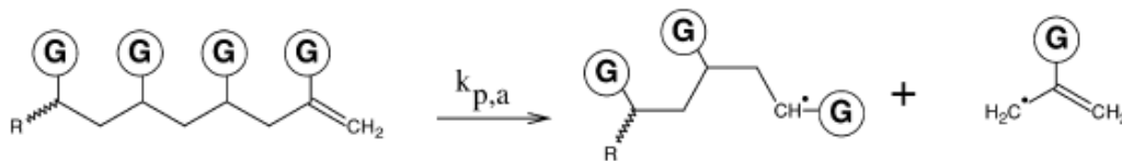
Figure 3-6 Sketch of end chain scission reaction in plastic pyrolysis [95]
