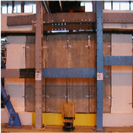
(a) Multi-panel super-assembly representing part of the precast concrete hollow-core wall system in a warehouse building.
