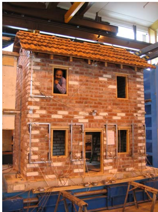
Figure 2: Model building on the shake table during testing in the longitudinal (E-W) direction
