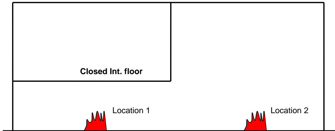
Figure 28: Schematic diagram of a firecell containing a closed intermediate floor and fire locations (section view)
